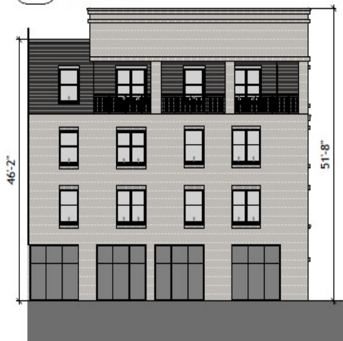
6 ELEVATION - BUILDING 100 - POOL COURTYARD NORTH A3-02 1/16" = 1'-0"
