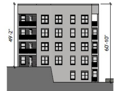
10 ELEVATION - BUILDING 100 - EAST A3-03 1/32" = 1'-0"
