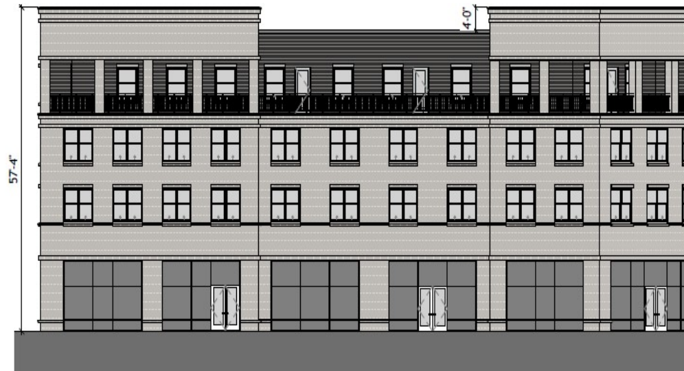
5 ELEVATION - BUILDING 100 - SOUTH A3-02 1/16" = 1'-0"
