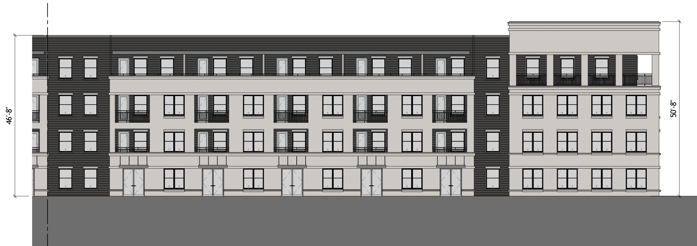
11.2 ELEVATION - BUILDING 200 - EAST 2 A3-07 1/16" = 1'-0"
