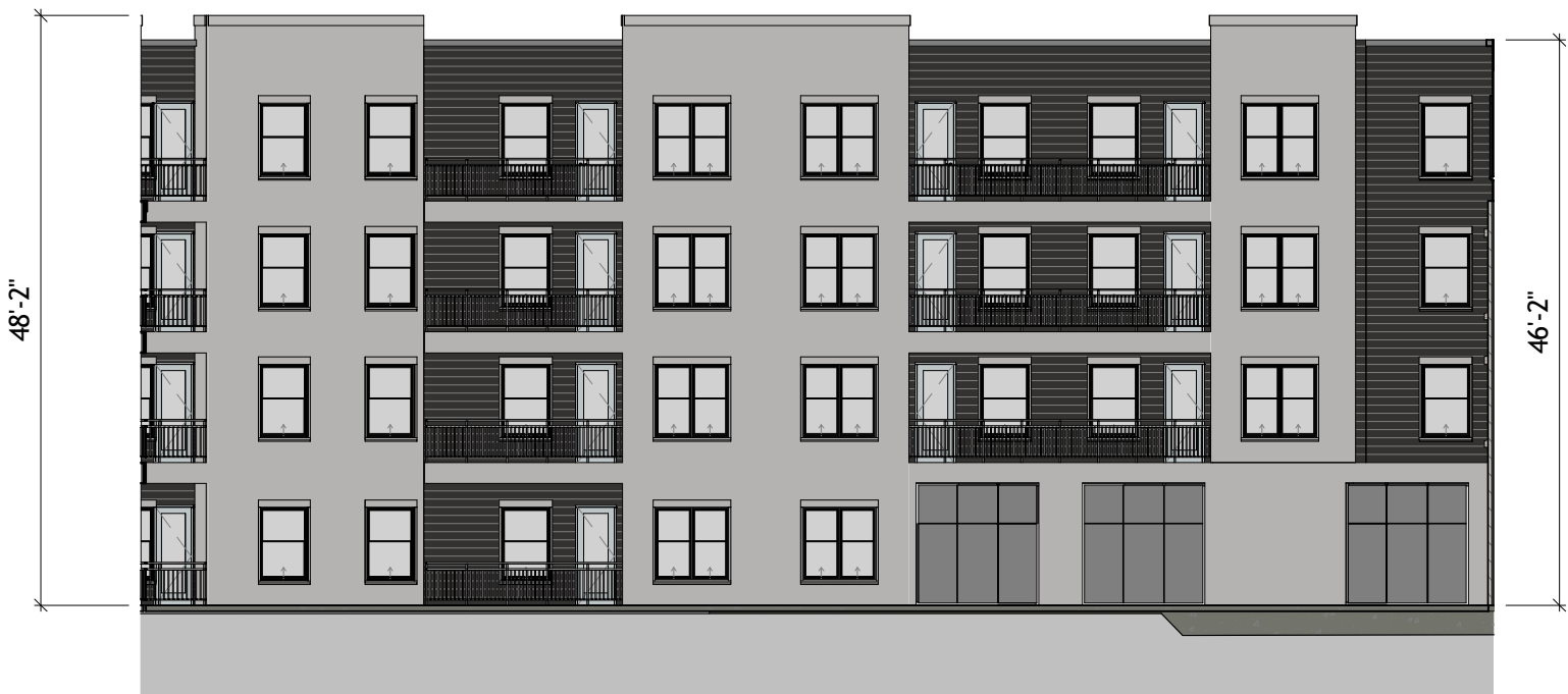
7 ELEVATION - BUILDING 100 - POOL COURTYARD WEST A3-02 1/16" = 1'-0"
