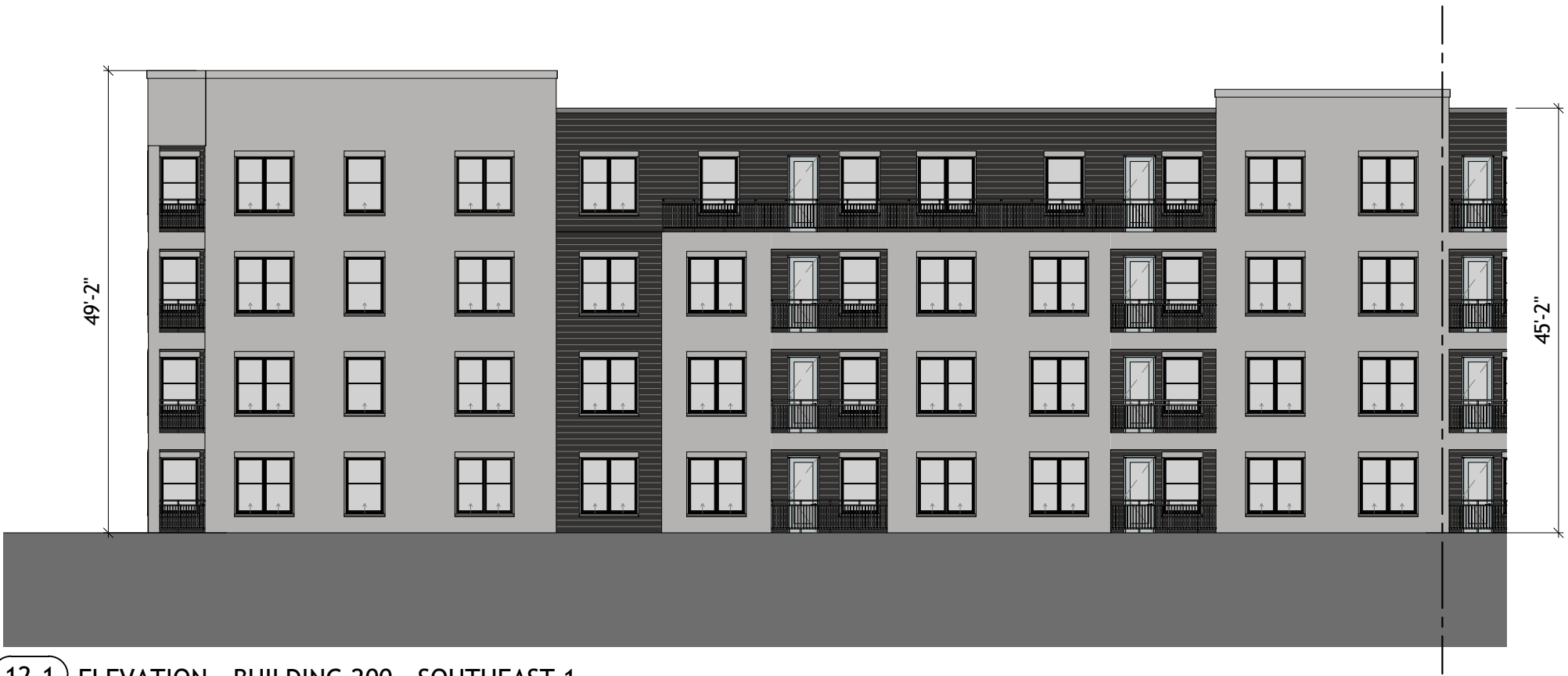
12.1 ELEVATION - BUILDING 200 - SOUTHEAST 1 A3-08 1/16" = 1'-0"
