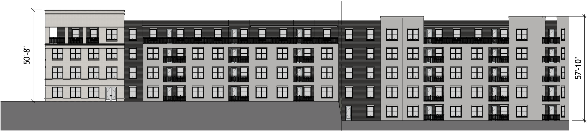
1 ELEVATION OVERALL - BUILDING 200 - WEST A3-10 1/32" = 1'-0"
