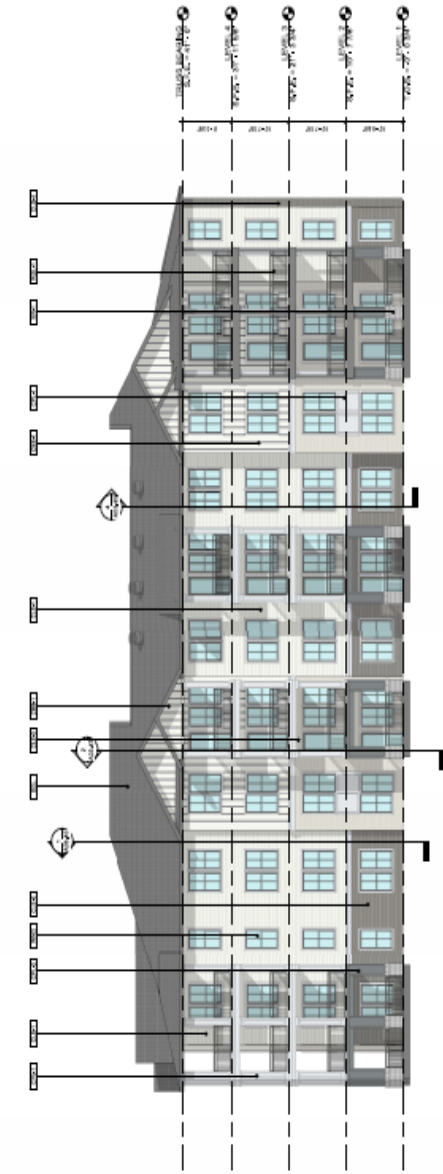
1 BUILDING TYPE 460 L SIDE 1 ELEVATION 1/8" = 1'-0"
