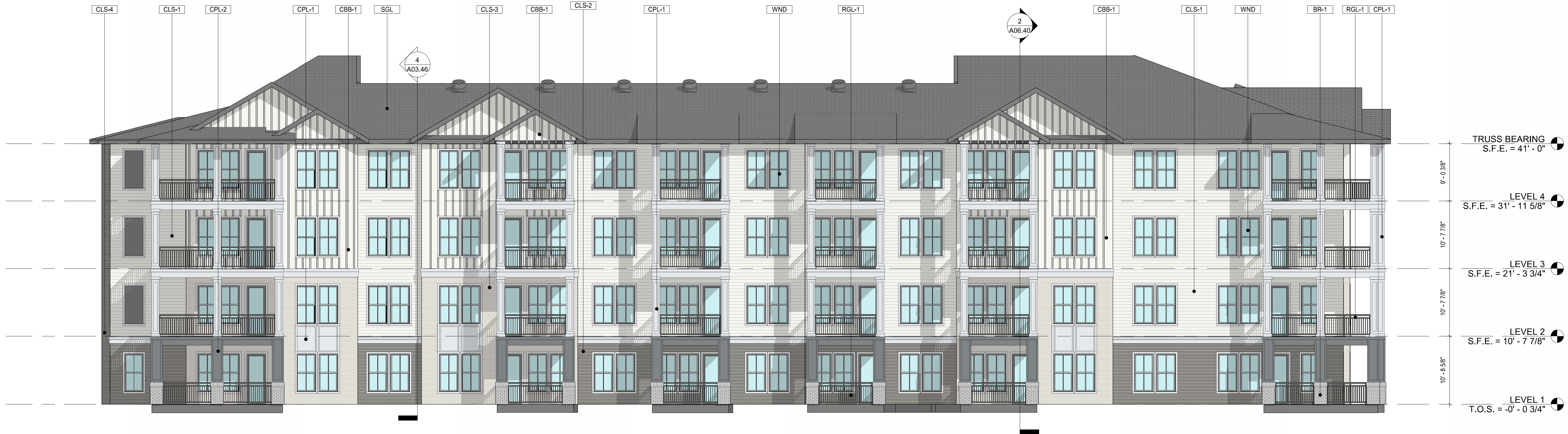
2 BUILDING TYPE 460 L REAR ELEVATION 1/8" = 1'-0"
